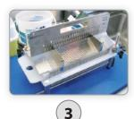
Slide side boards through grooves to hold specimen firmly in place
