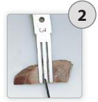
Cut other side of the central fork to obtain a pre-set thickness specimen.
