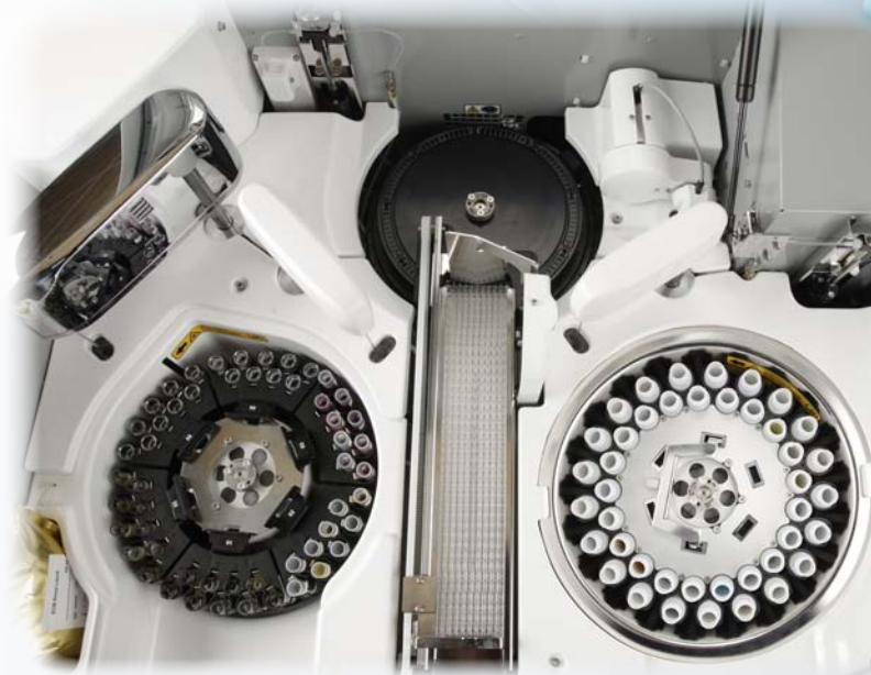
Indiko Plus has a sample disk for 54 samples : 9-pos. sample racks, max 6 racks.
