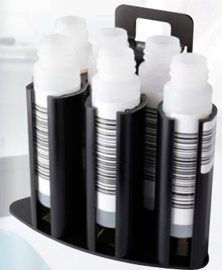
6-positions reagent rack used in Indiko
