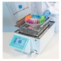
3 Eliminate excess reagent by placing filtering cage on the built-in front hinges.
