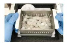
7 Up to 25 cryovials can be simultaneously frozen.
