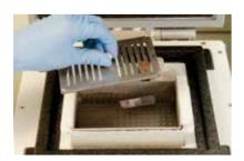
4 Set the metal plate in the tank. Place the metal cover on top of the fluid tank.
