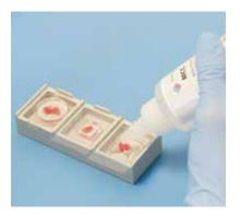
Fill the cryomold with the Milestone MCC compound.
