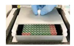
The rack holder accepts 24/48/96-well plates. The procedure is the same for random biospecimens.
