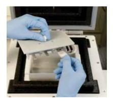
7 Slide the cryomolds from the holder.
