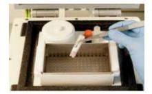
3 Set the cryovial in the random sieve-type holder and immerse it in the fluid tank.
