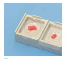
Set the cryomolds in the holder and place the specimens in each cryomold.
