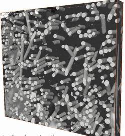
3D reconstruction of an automotive oil filter casing (polymer/glass fiber composite)
