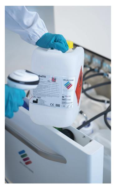
The LOGOS One EVO reduces the risk of water contamination and carry-over via **two separate paths to handle water-based and alcohol-based solutions**. This feature extends the lifetime of the reagents whilst securing the preservation of the specimens. LOGOS One EVO provides high quality processing for all tissue types, including SuperMega cassettes and fatty tissues.
