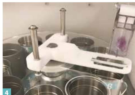
4 After 2'17" in high quality mode (in 3'51" in ultra-quality mode) six slides are processed/stained, ready for coverslipping and examination.
