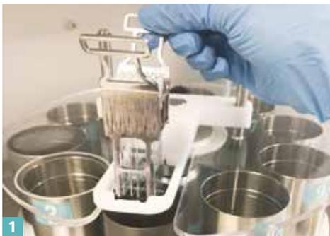
1 Position the slide rack over the FineFIX processing vessel.
