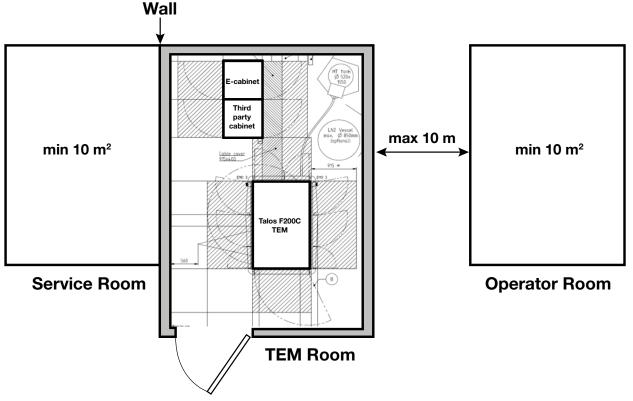
Figure 3. Recommended room layout for Talos F200C TEM. The third party cabinet is needed only for an optional energy filter or other special configurations. The required room dimensions are then extended to 5.77 m x 3.90 m (18.9 x 12.8 ft).
