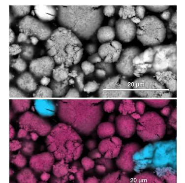
ChemiSEM image of an NCM battery electrode. The contribution of the EDS information given by ChemiSEM Technology highlights the presence of Zr contaminants in the matrix of the electrode. This would have otherwise gone unnoticed, as the compositional contrast in the CBS image in this case is insufficient to see the presence of unknown elements.
