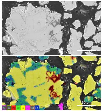
ChemiSEM image of a cement sample, acquired in low vacuum with a pressure of 150 Pa. The image shows the distribution of different phases such as periclase (MgO) in red and ferrite in green/blue (Ca<sub>2</sub>(Al,Fe)<sub>2</sub>O<sub>5</sub>). The yellow phase is a mixture of both Ca and Si, so it is either alite (Ca<sub>3</sub>SiO<sub>5</sub>) or belite (Ca<sub>2</sub>SiO<sub>4</sub>). The image also shows the presence of an unexpected contaminant (in pink), which is sulfur-rich.
